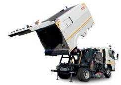
The special high tipping technology allows **raising the debris hopper to 1.50 m** and emptying it in a provided container.
