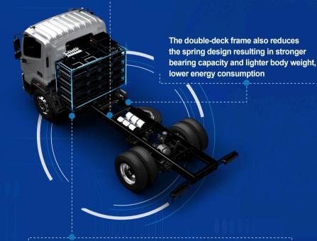
Battery back design to improve vehicle safety chassis reserved with more space to adapt to more special restructuring
